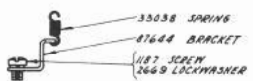
87593 SET OF PARTS FOR MECHANICAL END OF LINE INDICATOR. (INCLUDES ALL PARTS SHOWN ON THIS PAGE)
