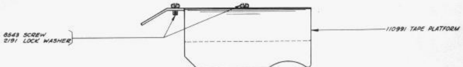
TAPE PLATFORM USED ON FRXD3 AND 4
