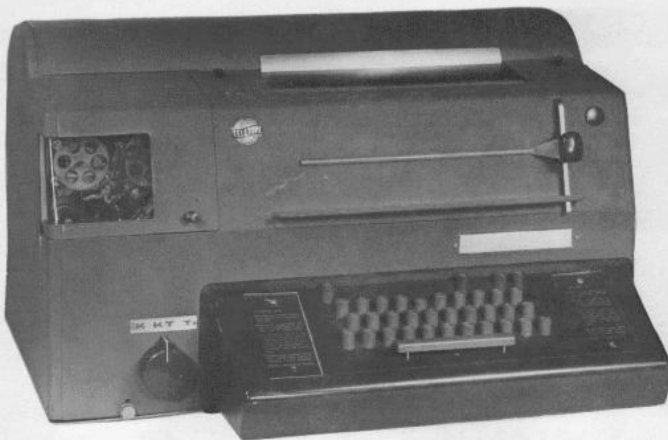
MODEL 28 AUTOMATIC SEND-RECEIVE KEYBOARD BASE (LAK) WITH TYPING PERFORATOR (LTPE) AND COVER (LBPC)
