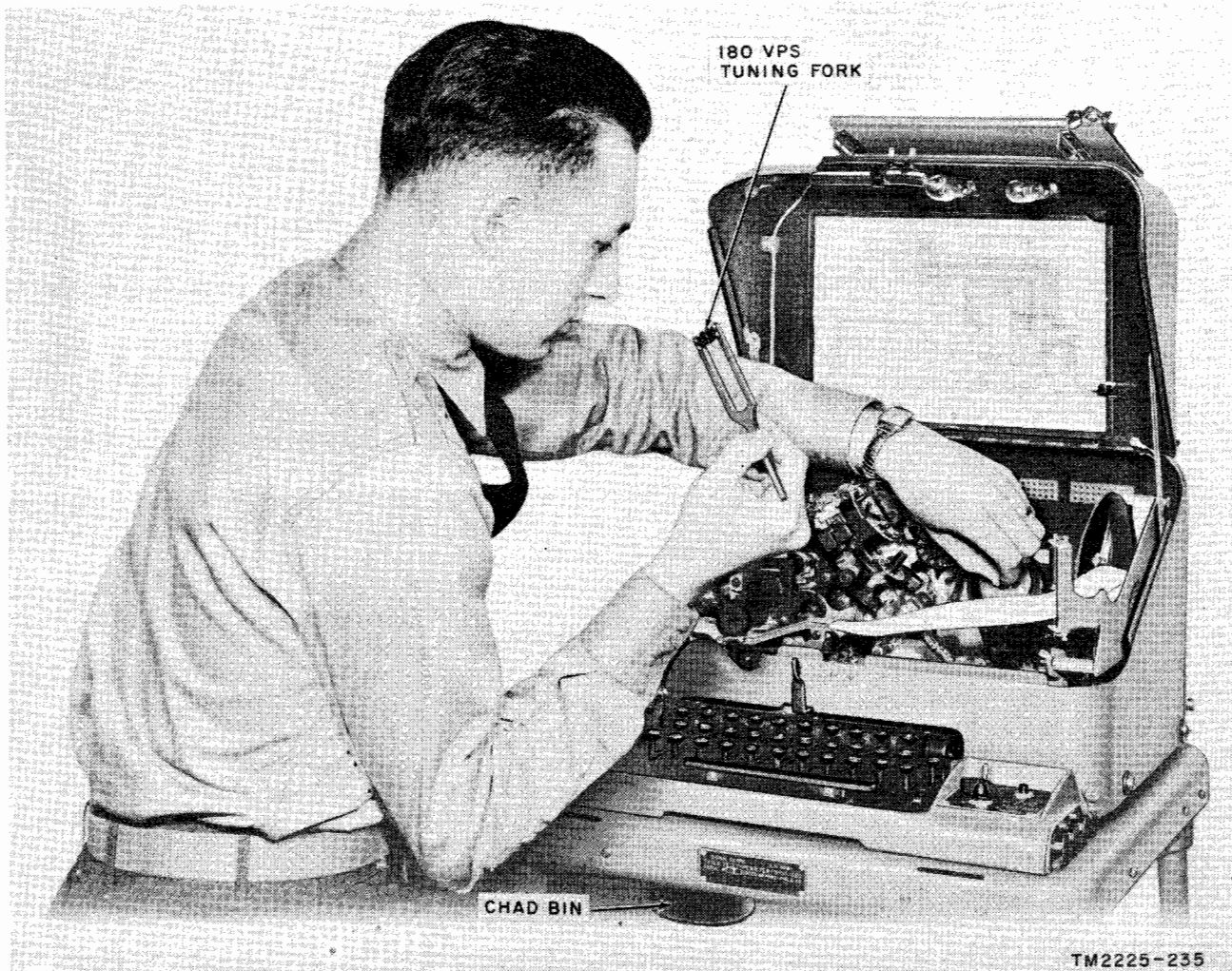
Figure 2-6. Checking motor speed.
