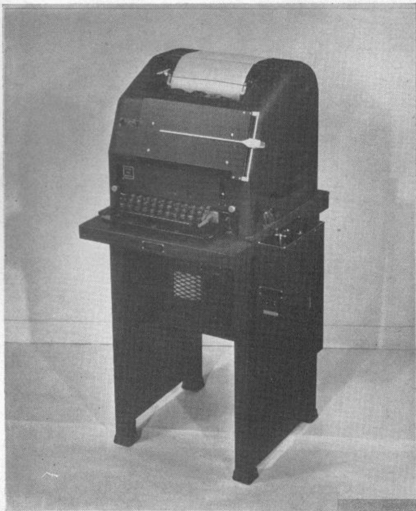
Fig. 1—SE200-type control unit mounted on a table with a 15-type teletypewriter.
