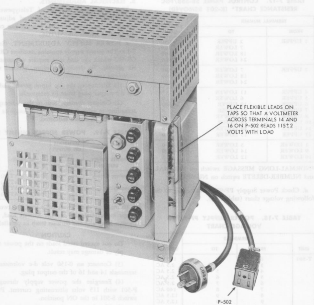
Figure 7-1. Power Supply PP-987/U, Adjustments
