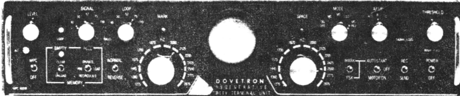
THE MPC-1000R REGENERATIVE RTTY TERMINAL UNIT
