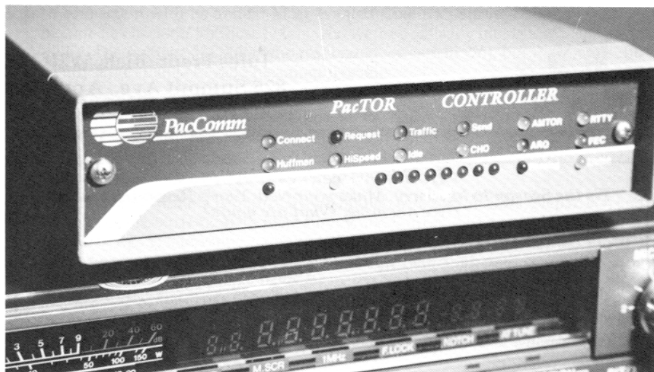
PacComm's PacTOR Controller, Front View
