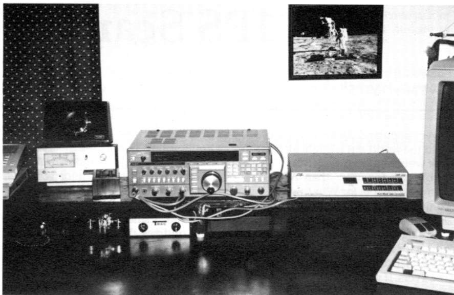
Picture 2: A look at my station shows the DSP-1232 next to my YAESU FT-736R transceiver. On the left are rotor controls for my tracking antennas and on the right is my 18-inch monitor for nifty graphics.
