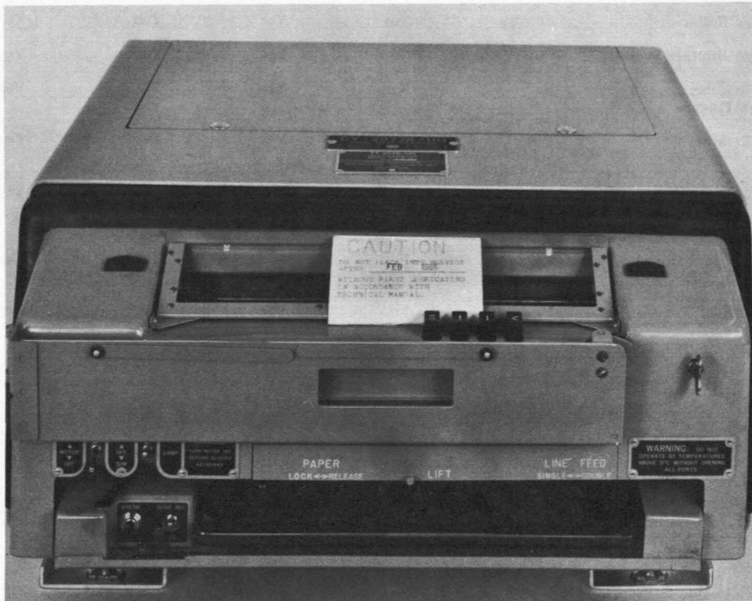
Figure A2-1. Front View of Teletypewriter TT-299B/UG Showing Calendar Lubrication Requirements
