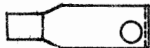
B80 0.144" HOLE CENTER LOCATED \frac{1}{8} " FROM END & \frac{1}{8} " FROM SIDE. SEL. SW.
