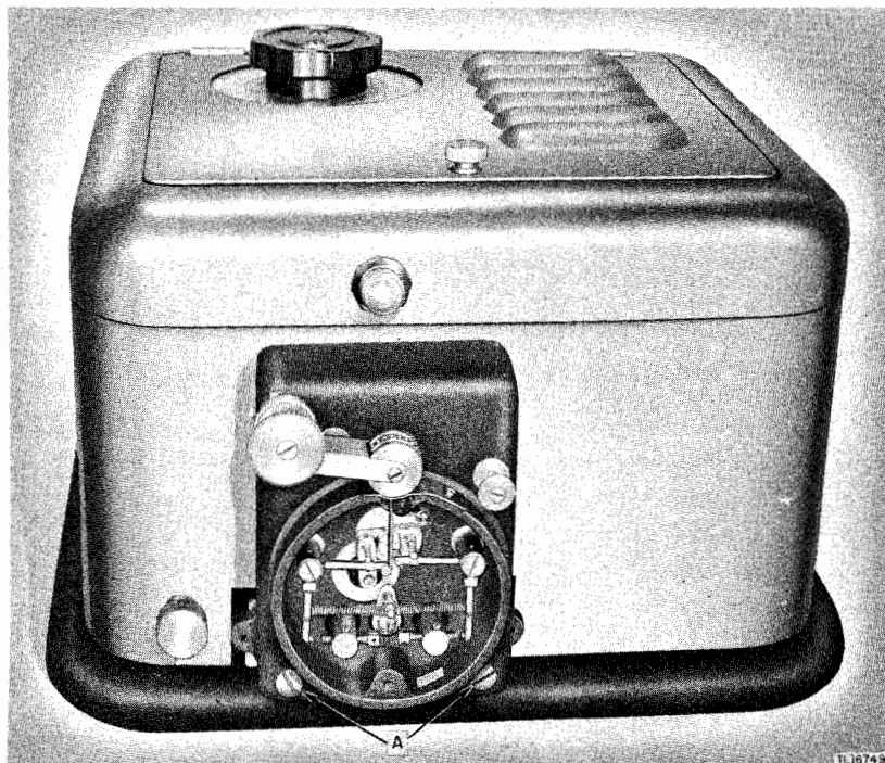
Figure 17. Auto head and drive unit, showing first step in disassembly.
