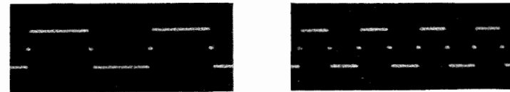
CATHODE-RAY OSCILLOGRAMS SHOWING REVERSALS AT 120 W.P.M. (LEFT) AND AT 240 W.P.M. (RIGHT). NOTE THE SHORT TRANSIT TIME AND THE COMPLETE ABSENCE OF REBOUND.
