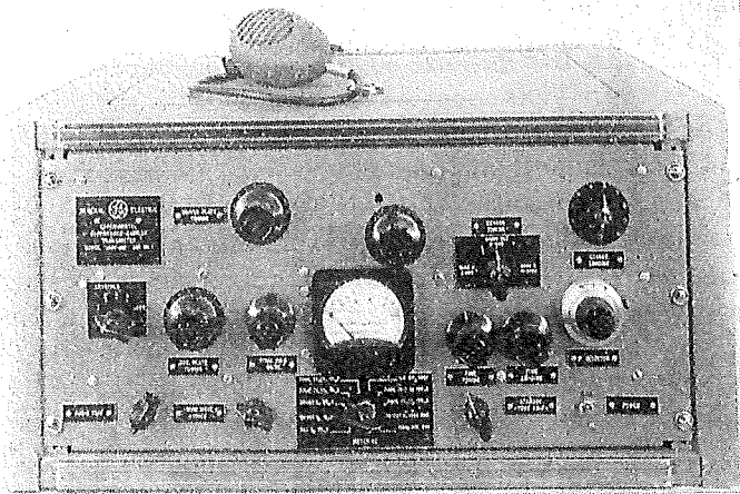
Fig. 5—The AN/FRT-29 (XW-1) suppressed-carrier AM transmitter.
