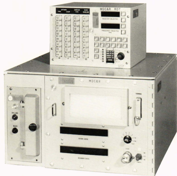
Figure 1 — Modular data collection and recording unit and remote data terminal.
