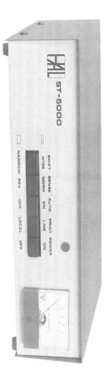
The HAL ST-5000 Demodulator provides reliable RTTY performance on both HF and VHF bands. A hard limiting front end, active discriminator, and active detector make this unit a big value. Standard features include 170 and 850 Hz shifts, normal or reverse sense, autostart, built-in loop supply, an audio tone keyer, and RS-232 input and output for connection to computer I/O ports. The ST-5000 is available in either standard 2125 Hz MARK (High Tone) or 1275 Hz MARK (Low Tone) versions.
